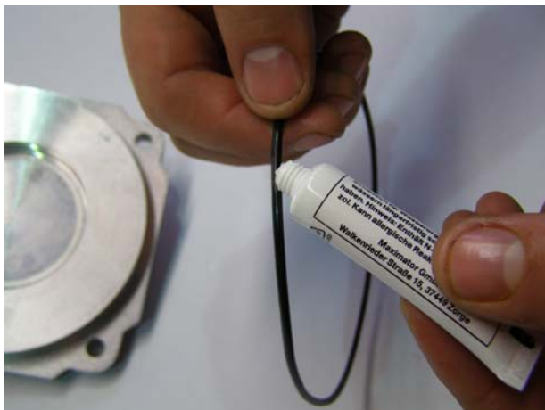
Grease and place the o-ring (item 9) into the bottom cap (item 46).
