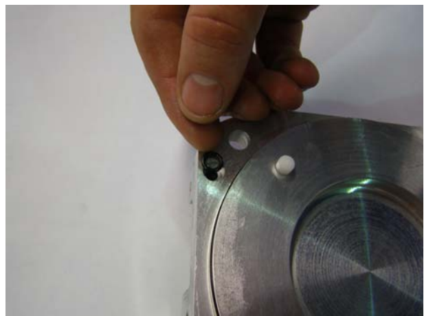
Grease and place the o-ring (item 9) into the bottom cap (item 46).
