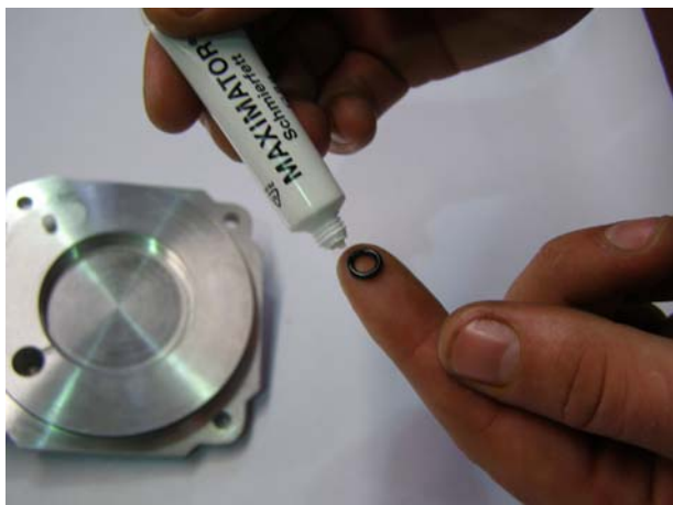
Grease and place the o-ring (item 9) into the bottom cap (item 46).
